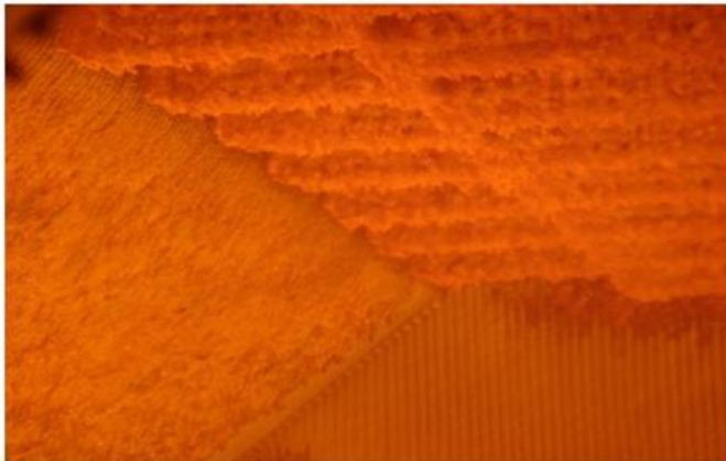
Figure 4.1 Unit slagging with 90% co-firing of straw
