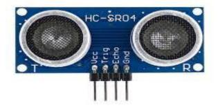
It works like this first a sensor sends a beam of sound for some time and then receives the sound back after it reflects it from any obstacle. Basically, it records the time in milliseconds during which ultrasonic sound has been sent and received. The pulse function is used for this purpose. But in this, we'll use some manual commands to control the Ultrasonic sensor.
