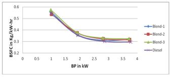
Figure 2. Brake Specific Fuel Consumption V/S Brake Power
