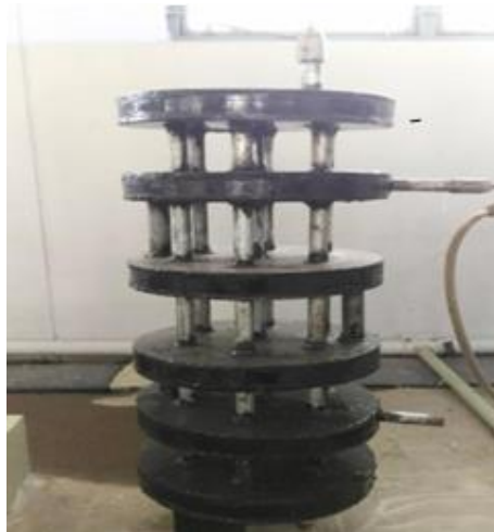
Fig 6 Model of carbon etched heat exchanger
