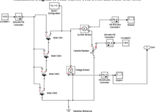
Simulation Diagram of Solar cell for both Boost and Buck Converter
