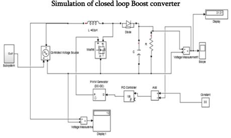
The output voltage of boost converter is shown in the figure below. The output voltage value is set as reference value in the constant block and compared with the actual output of boost converter taken as reference and given to Integral controller. Then the output of controller is given to the PWM generator. This generated pulse is given to the MOSFET.
