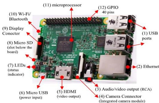
Fig. 1. Raspberry Pi 3 components.
