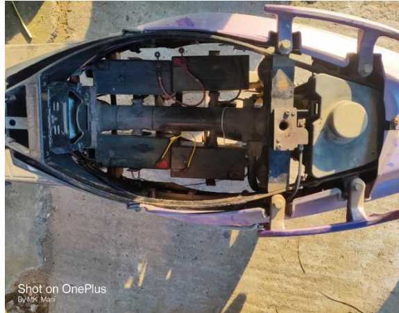
Fig. 12: Internal wiring connection of battery and motor
