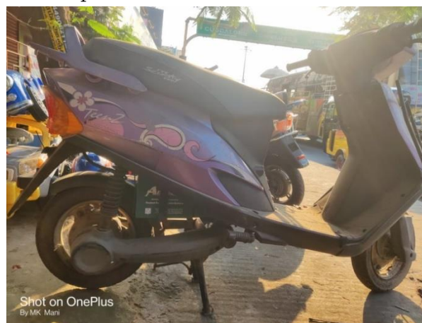
Fig 11: Prototype model showing Hub motor and Li Ion battery
