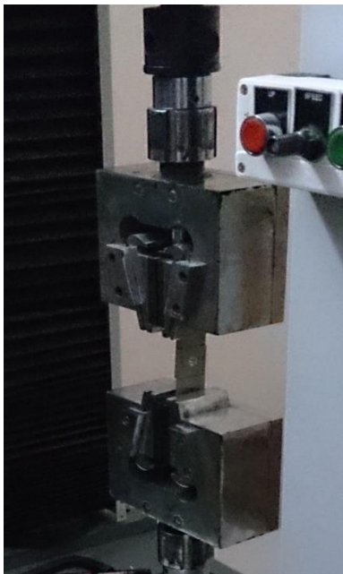
Fig. 6. A Photograph of lap shear test
