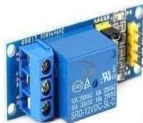
Fig3.4.a Relay Driver Unit
