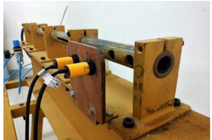
Fig.3.1 IR sensors mounted near the gun barrel
