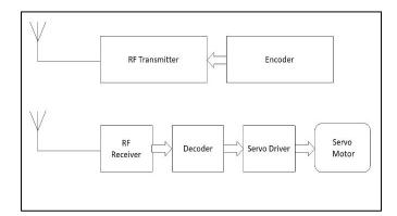
The Transmitter sends signal to the receiver when the transmitter is in the range, receiver receives the signal and send it to the microcontroller which then sends signal to the Servo motor and relay. A servomotor (or servo motor) is a rotary actuator or linear actuator that allows for precise control of angular or linear position, velocity and acceleration. We're using servomotor to unlock the Door of the cabin and relay to open and close the circuit.
