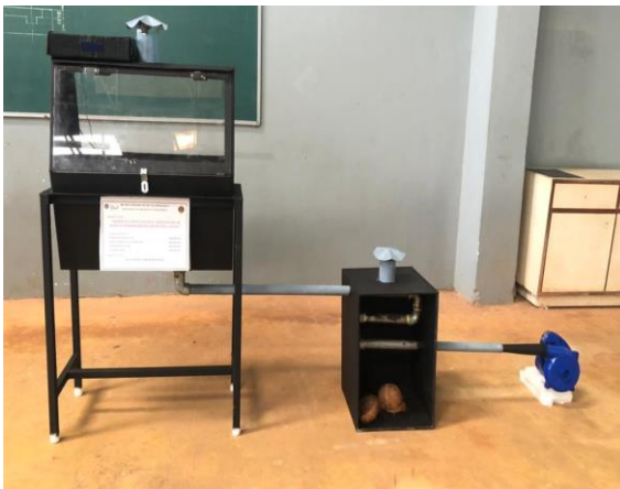
Fig. (7) Assembled Parts of Artificial intelligence assisted solar biomass hybrid dryer for drying cocoa
