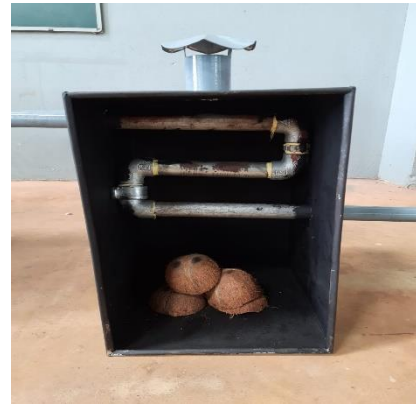
Fig. (4) Biomass Chamber
