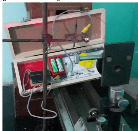
Figure 2. Production of LASER beam using Solar energy or cell for determination of wavelength.
