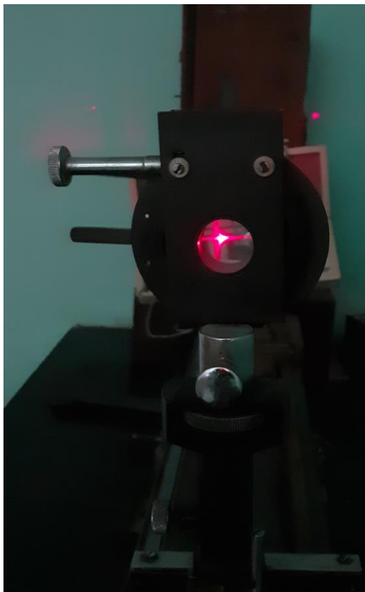
Figure 4. LASER beam falls on grating, it is generated from a Solar unit for determination of wavelength.
