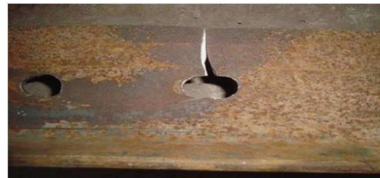
Fig. 4.1 Partial net section ruptures, with small eccentricity
