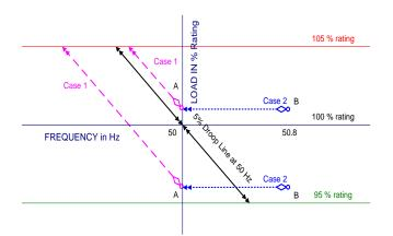
During the frequency rise from 50 Hz to a higher value, Load reduction signal is released up to 5 % as per the droop characteristics.
