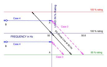
When the frequency is more than 50.8 Hz, the existing feature of Isolated Grid will take control of the turbine.
