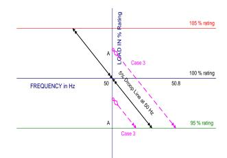
When the frequency rises from 49 to 50 Hz, Load reduction signal should be blocked.
