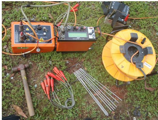
Figure 2: Tools and equipment used in electrical resistivity imaging
