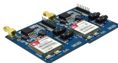
Figure 7 : GSM AND GPRS module
