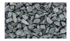
The coarse aggregates, ranging in size from 8 mm to 40 mm, are collected and thoroughly washed. The amount of water that leaks out depends on the size of the aggregate used. It is gravel and crushed stone that is mostly retained on the 4.75 mm screen. Size of aggregates used: 20 mm to 40 mm.
