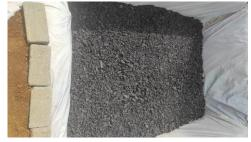
The well sized and shaped char product is placed over the geotextile layer. This charcoal has the ability to absorb the toxins and pollutants present in the wastewater, resulting in purification of the water.
