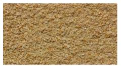
The fine aggregates, ranging in size from 2 mm to 4.75 mm, are collected using sieves and washed. The size of the particles leads to an increasing proportion of voids, which increases the permeability of the water. They
