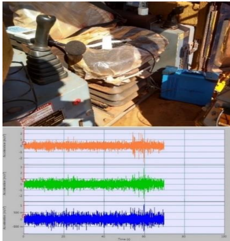
Figure 11: Vibration values Measurement on Operator's seat
