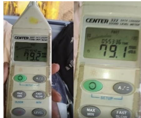
Figure 10: Sound Pressure Level Measurement at Operator’s Position
