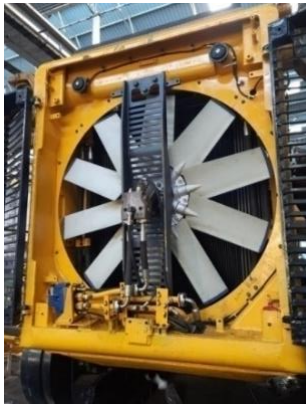
Figure 8: Cooling fan mounted in front of cooling system
