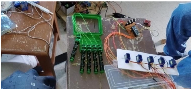
Figure 6. Robotic arm with 5servo motors
