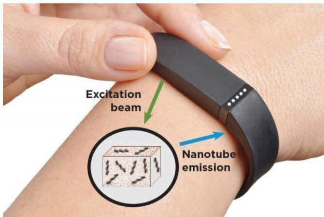
Fig. 6 A small device worn on the wrist could send light into the sensors (excitation beams) and analyze the light coming back out (nanotube emission) to provide constant updates [21].
