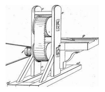
The Hybrid Band saw cutting machine is a type of cutting machine that has been in use for over a century. Its popularity in the industry can be attributed to its versatility, speed, and accuracy. The first Hybrid Band saw cutting machine was developed in the mid-1800s and used a continuous blade loop made from a thin strip of steel. The blade loop passed over two pulleys,
