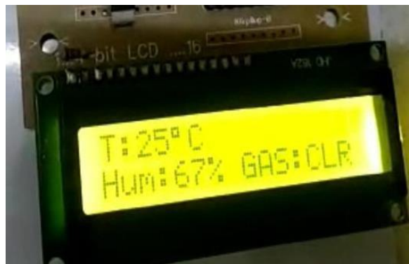
Fig.5. Output on LCD when gas is cleared
