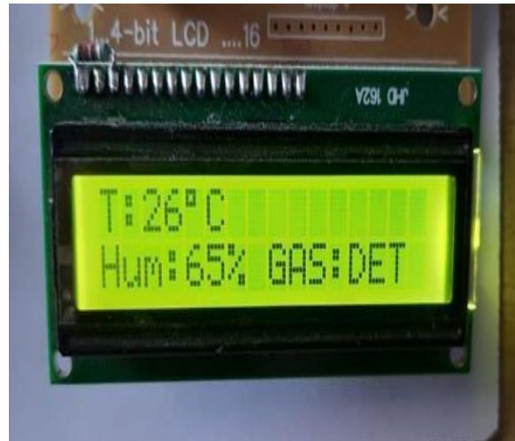
Fig.4. Output on LCD when gas is detected
