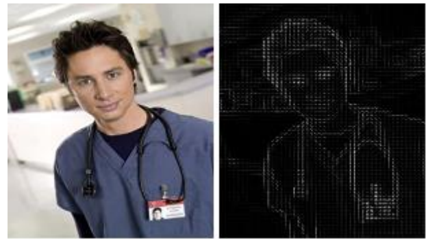
Figure 4. A sample of an original image and its histogram of gradients
