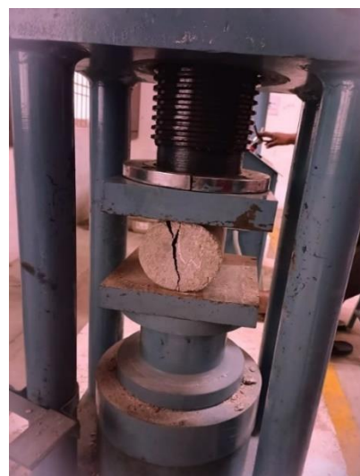
Figure : 4.2 Split tensile test
