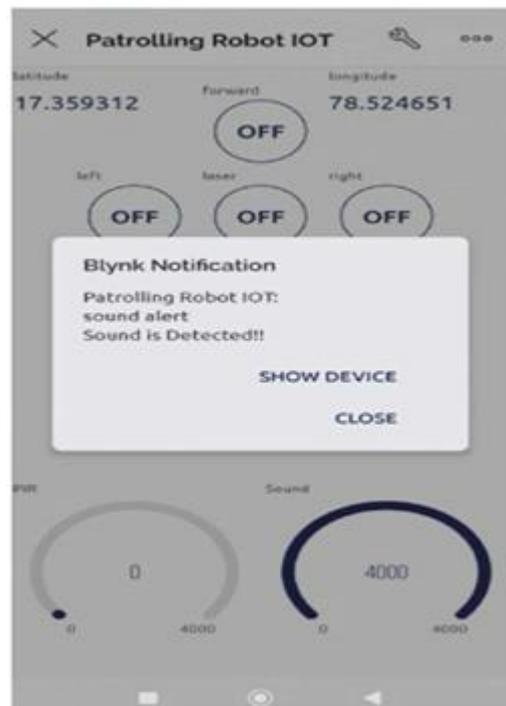
Fig. 7: Sound Sensor Alert
