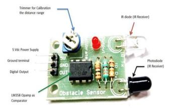
The IR sensor module consists mainly of the IR Transmitter and Receiver, Op-amp, Variable Resistor (Trimmer pot), output LED along with few resistors.
