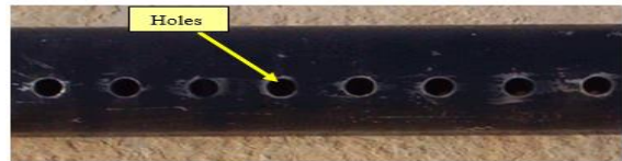
Figure 2a. Schematic diagram of the absorber of 20 holes of 20 mm diameter.
