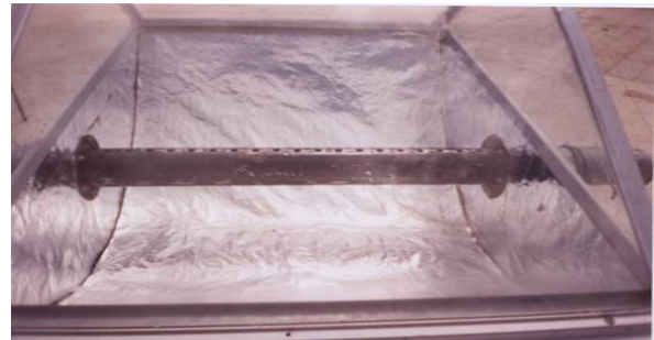
Figure 2b. absorber of 20 holes of 20 mm diameter of the evaporator
