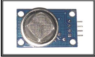
The gas sensor module consists of a steel exoskeleton under which a sensing element is housed. This sensing element is subjected to current through connecting leads. This current is known as heating current through it, the gases coming close to the sensing element get ionized and are absorbed by the sensing element. This changes the resistance of the sensing element which alters the value of the current going out of it.
