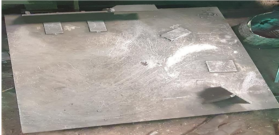
Figure 13: Support plate for prevention of miss location and distortion the workpiece
