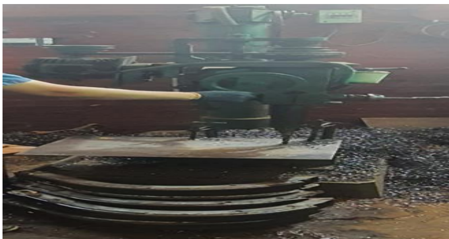
Figure 15: Piercing hole after forming by introducing drilling machine
