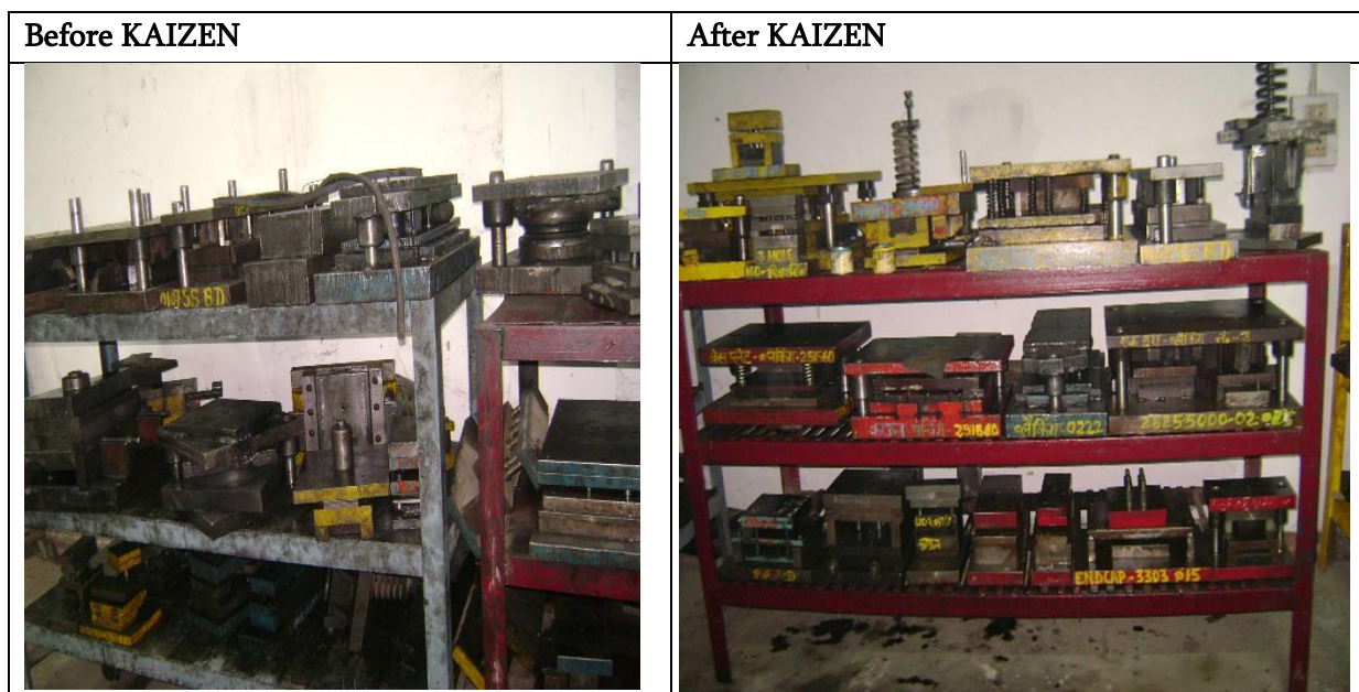
Figure 4: Easy Identification & Traceability Improved by using KAIZEN
