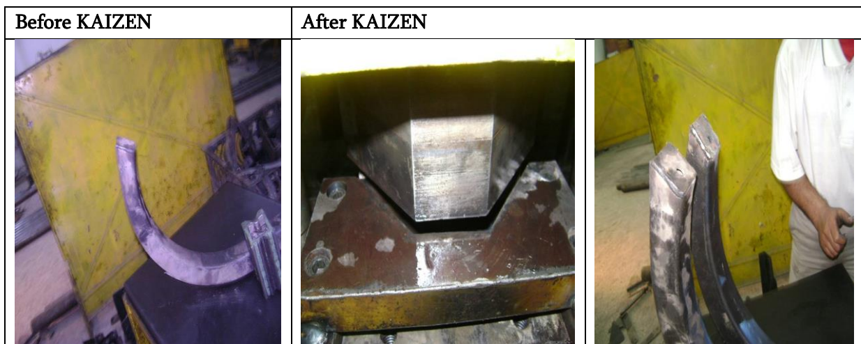
Figure 7: Improved the Die angle by using KAIZEN
