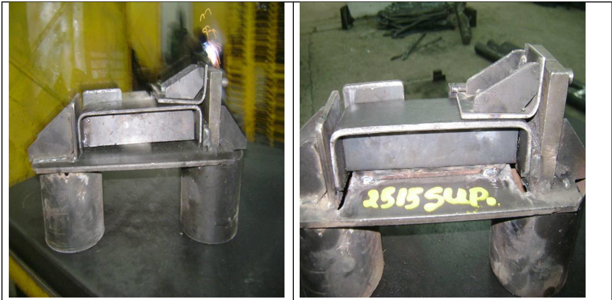
Figure 9: Improved in the Slot made & strip welded by using KAIZEN
