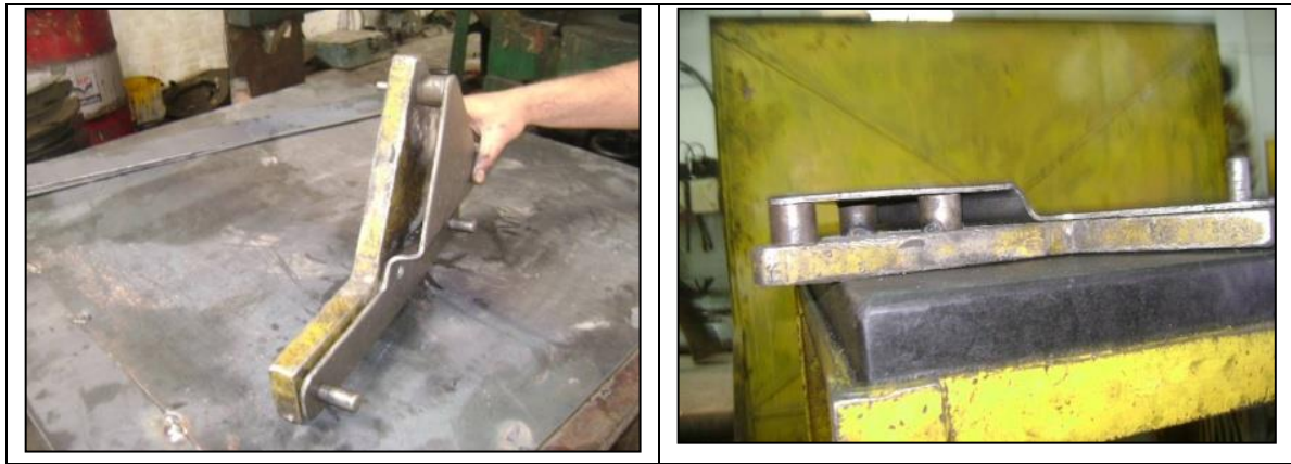
Figure 10: Improved in the Slot made & strip welded by using KAIZEN
