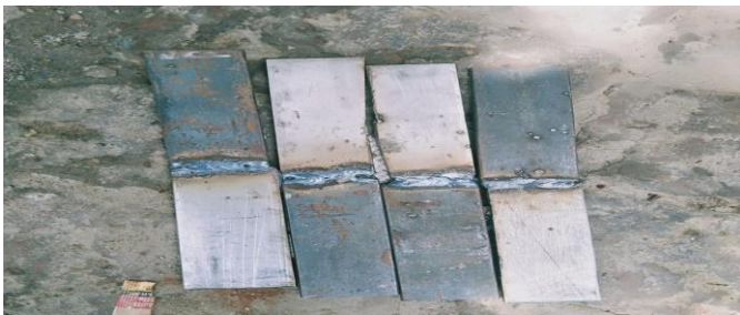
Fig-4 Test Specimen(Stainless Steel 304 and Mild steel)
