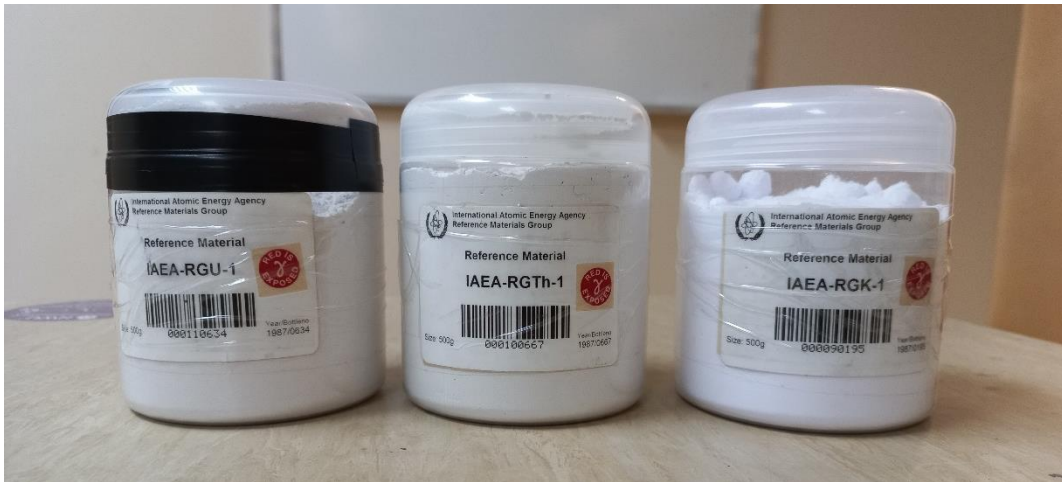
Figure 2 : The IAEA radiometric reference materials; RGU-1, RGTh-1 and RGK-1 for calibration of both energy and efficiency for HPGe detector at CARST.
