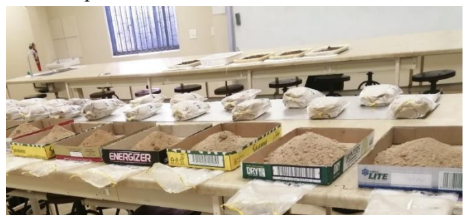
Figure 1: Packaged plastic containers and cartons used for spreading samples for drying out moistures.
