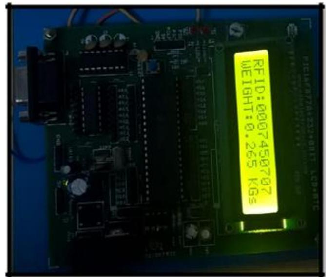
Fig.5. Displaying RFID and weight in LCD
