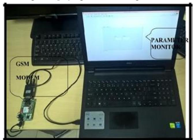
Fig.6. Software system interface at receivers End
