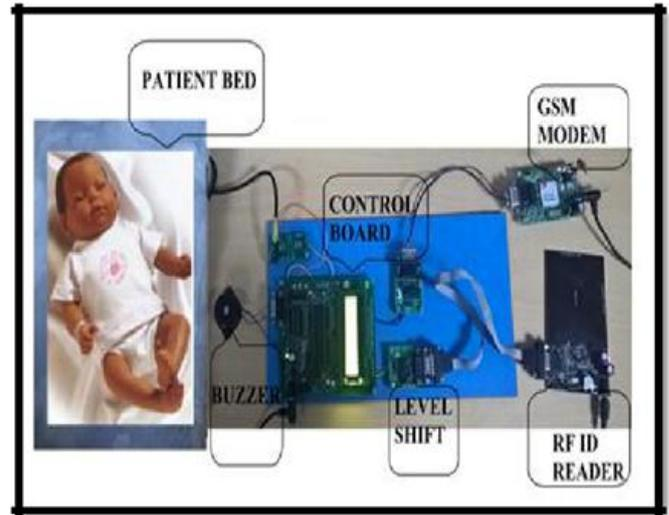
Fig. 4. Actual Implemented System in transmitter end
