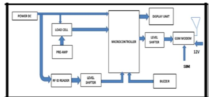
Fig. 1. Block Diagram of Transmitter Section
