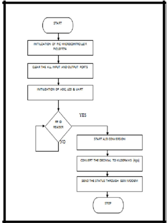
Fig.3. Flow chart for Transmitter section
