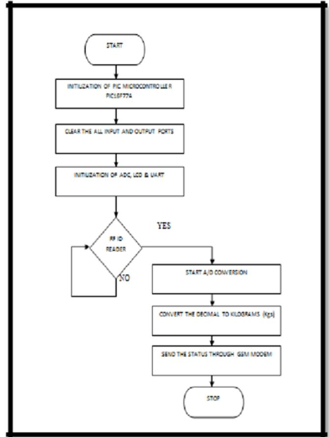
Fig.3. Flow chart for Transmitter section
