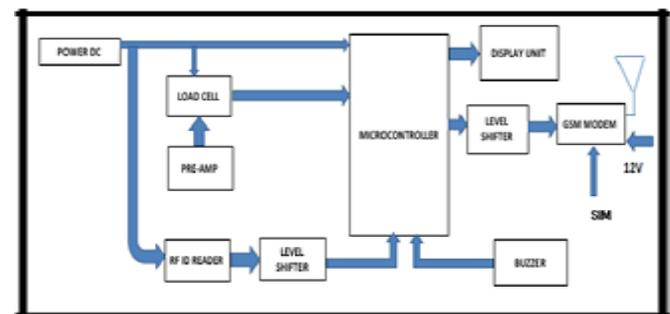
Fig. 1. Block Diagram of Transmitter Section
