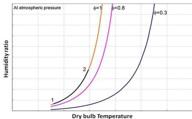
Fig 2.5 Closed-air open-water (CAOW) water-heated system on psychometric chart
