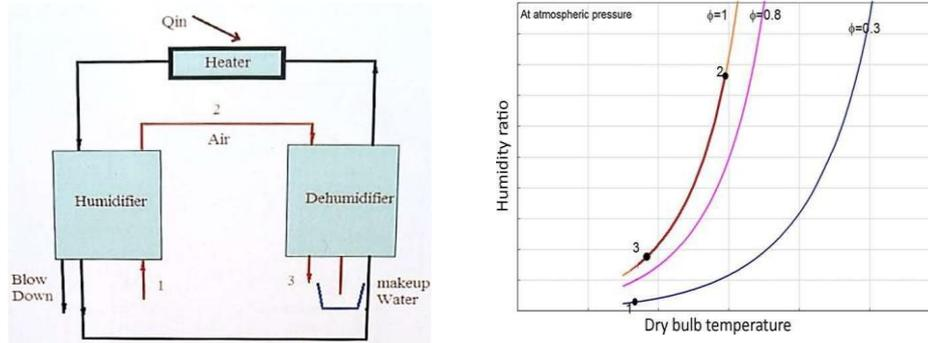
Fig 2.7 Closed-water open-air (CWOA) water-heated system
