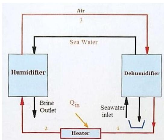
Fig 2.4 Closed-air open-water (CAOW) water-heated systems
