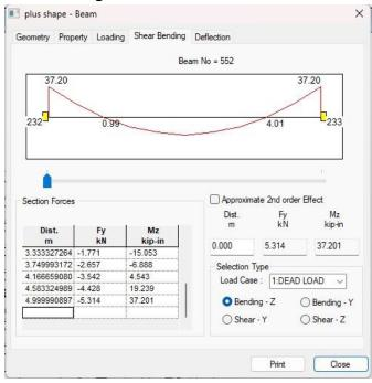
Shear Bending of Column
