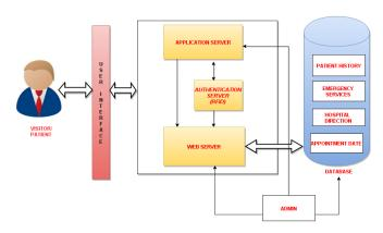
Figure 1: System Architecture
