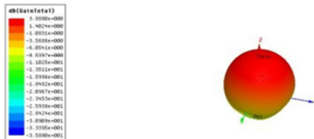
Fig 2(b) 3D radiation pattern of rectangular microstrip patch antenna with mica as dielectric material
