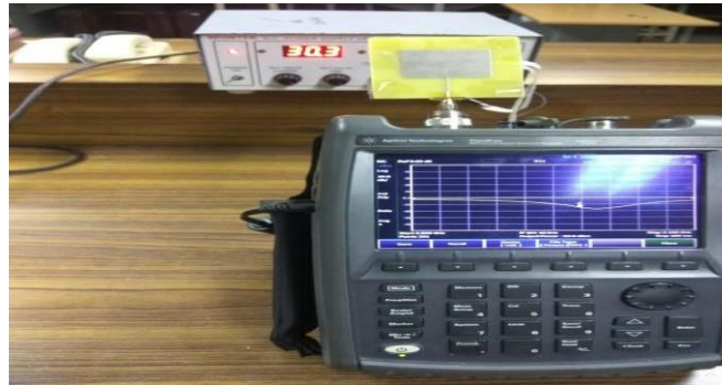
Fig 3(a) Experimental setup to measure the return loss of rectangular microstrip antenna with teflon material
