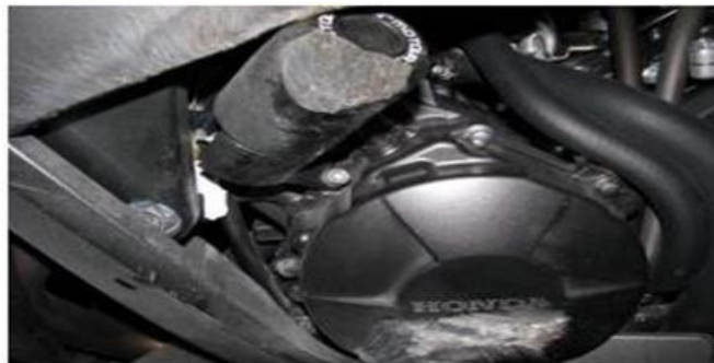
Fig 1 Damage engine case
