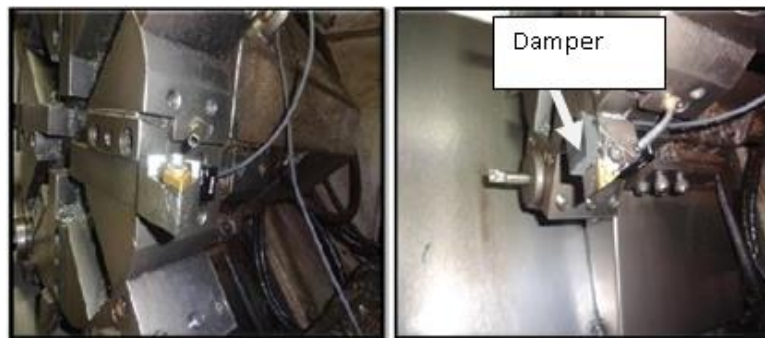
Diagram shows tool without and with damper
