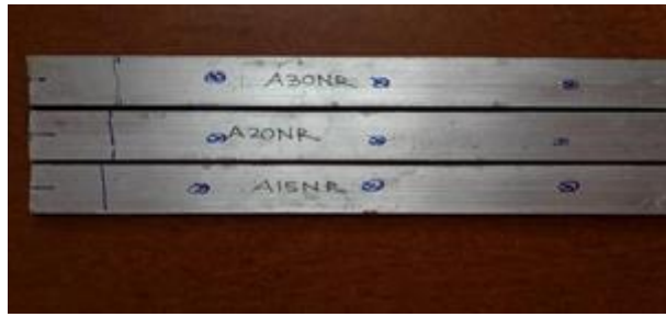
Fig. 11 Natural Rubber Beams
