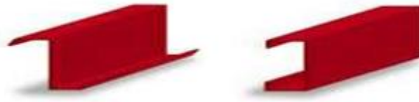
Figure2: Cold formed Z-sections
