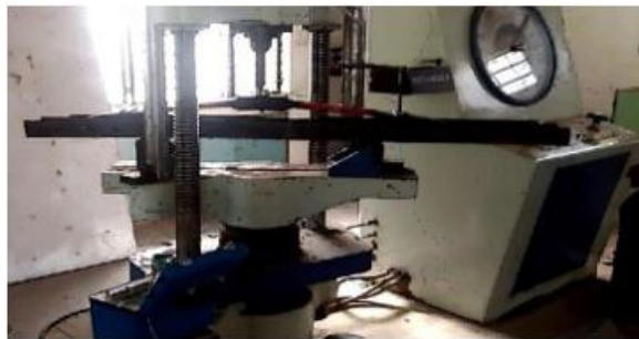
Figure3:Experimental Testing on Composite Leaf Spring.
