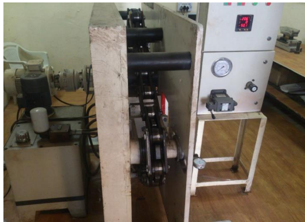
Figure1:Experimental set up to find elongation of chain on preloading and length measuring machine
