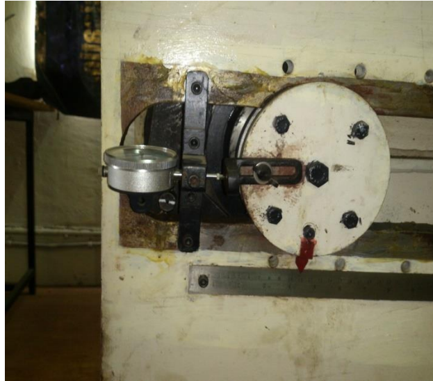
Figure2:Dial gauge location for measuring elongation of chain
