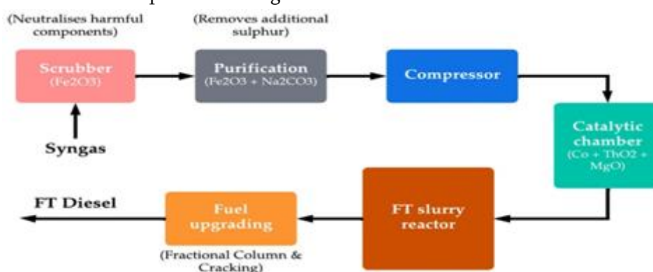
Fig 12. FT diesel production from syngas - Typical Fischer-Tropsch process
