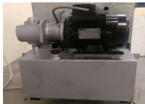
Figure 9: Hydraulic power pack
