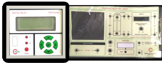
Fig. 3. Picture of Over/Under Frequency Relay
