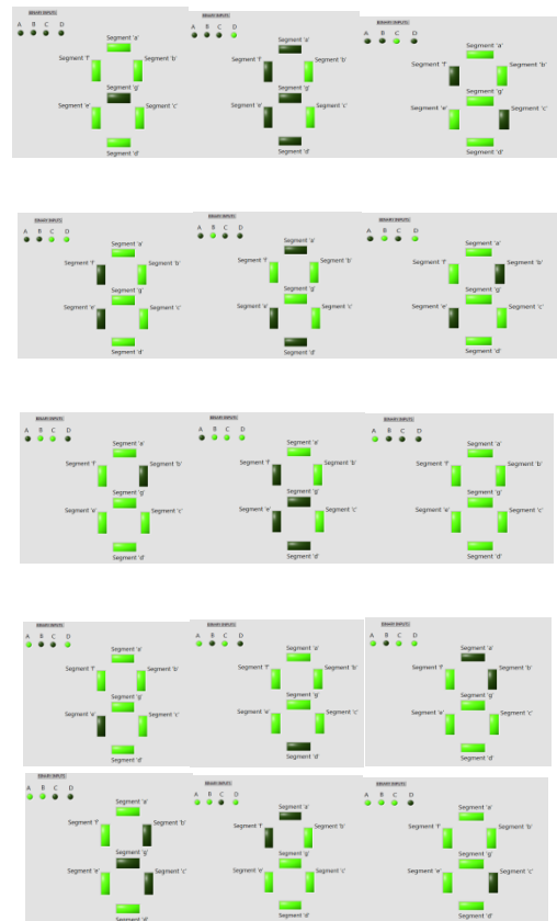
Figure 6. Decimal/Hexadecimal Display from (0 to 9, A, b, C, d, e)
