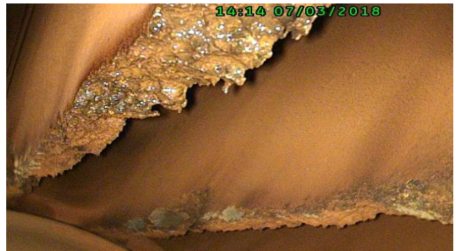
Figure 4 .vacuum pump impeller rotor damages due to cavitation
