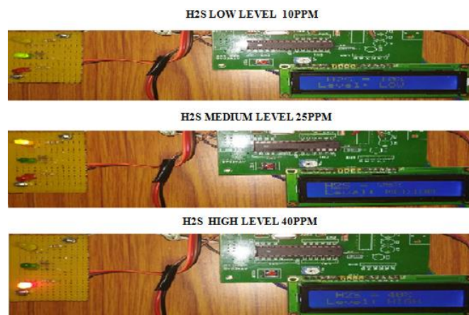
Figure 10. When the H 2 S gas reaches a certain level in drainage channel and display Hydrogen sulphide and level of gas. If Low level reached then LCD display shows the 10ppm , Medium level reached then LCD display shows 25ppm , High level reached then LCD display the level 40ppm and corresponding LEDs will glow as per the level of gas present inside the drainage channels.
