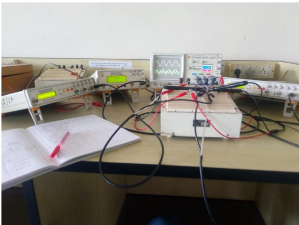
(b) Implementation of PAM-TDM circuit
