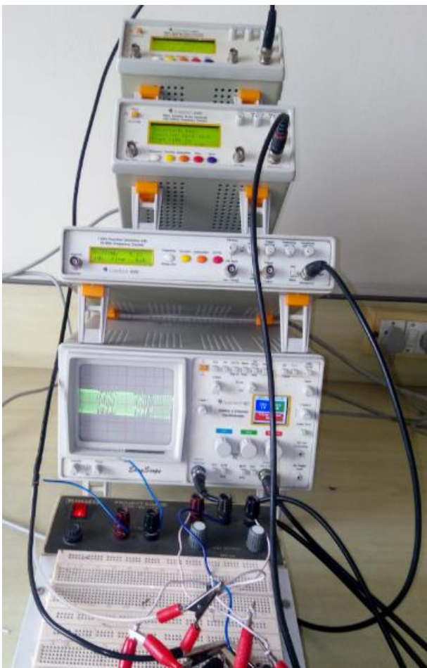
(b) FSK Implementation and Its Output Waveform Fig. 10. FSK Waveform Generation
