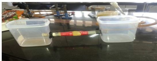
Figure 2. The Chambers Connected with the Salt Bridge
