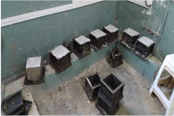
Figure 1. Casting of cubes
