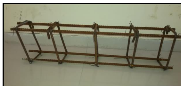
Photo 2. Cage of conventional beam section
