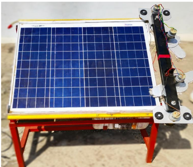
Figure 1. Front view of solar panel cleaning system
