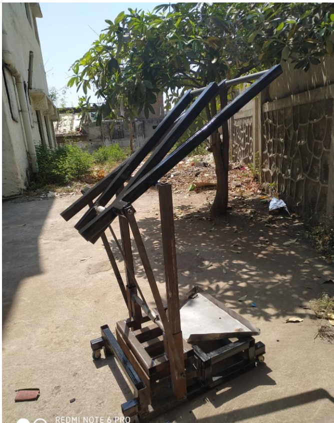
Figure 4. Brick moulding equipment.
