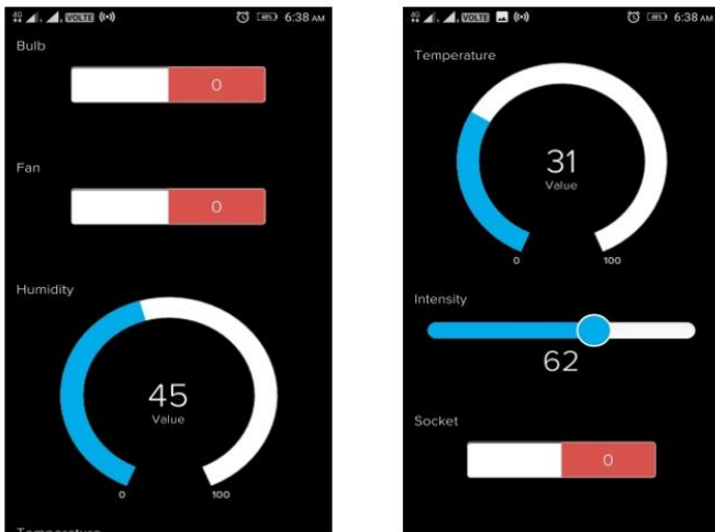
Figure 4 : GUI in android devices to control esp8266
