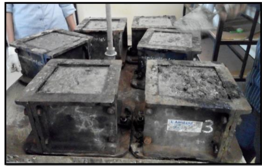
Photo 6. Compaction of cubes
