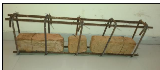
Photo 3. Cage of brick in filled beams section
