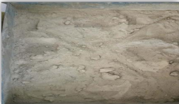
Figure 1. Coal Bottom Ash of Butibori Relience Power Plant
