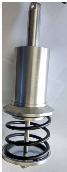
Figure 3. Actual electromagnetic Shock Absorber
