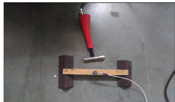
Figure 1. Experimental setup of simply supported beam using FFT Analyzer
