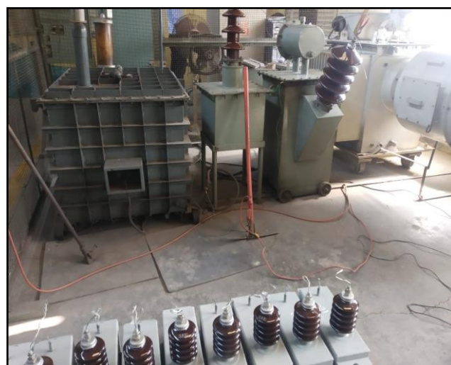
Figure 5. Voltage test of capacitors
