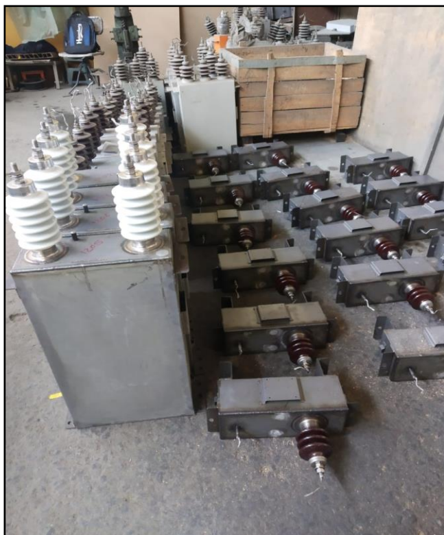
Figure 3. Winding and casing for capacitor banks
