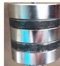
Figure 5. Stack of neodymium and iron core
