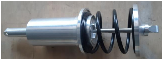
Figure 7. Electromagnetic actuator casing with spring.
