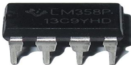
Fig.7.LM358-Single Supply Dual Operational Amplifiers
