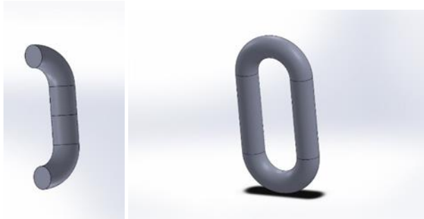
Fig 6. Non-weld model Fig 5. Link chain solid works model
