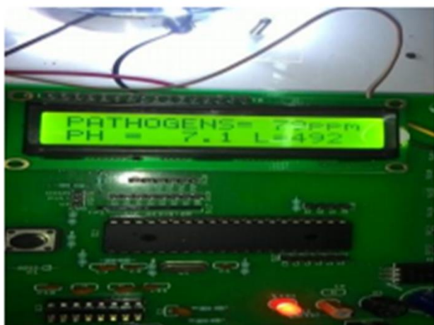
Fig 4 : LCD display of pH value for water sample
