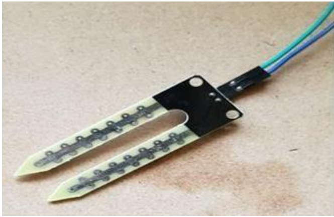
Figure 4: YL-38 Soil Moisture Sensor Module
