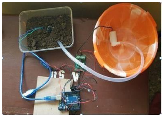
Figure 10: A Sample Test of the Designed Smart Irrigation System.
