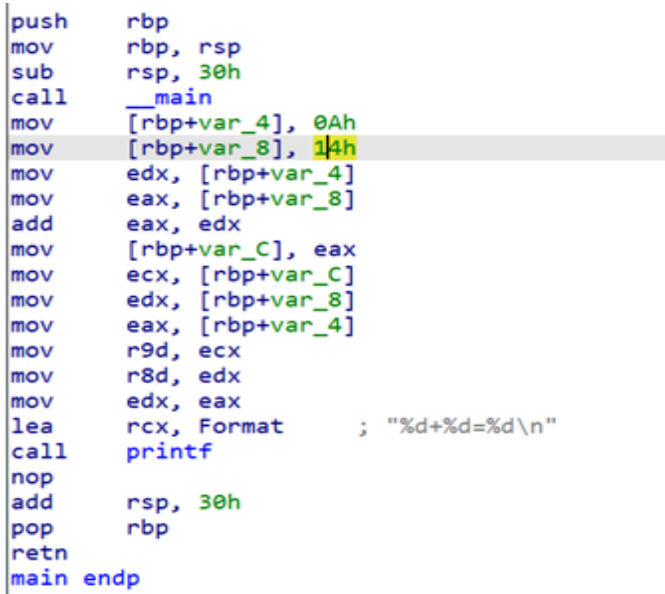
Fig. 2: Interactive Disassembler View of Prog
