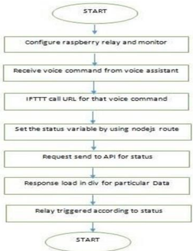
Fig.2 - Block flow of proposed model.
