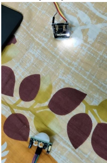
Figure 4. PIR-No movement detected
