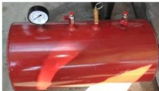
Fig 5. Compressed air tank[6]
