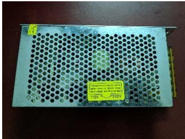
Fig 4.1. AC to DC Converter
